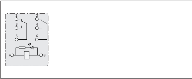
Connection diagram (bottom view) ZZ(B)
