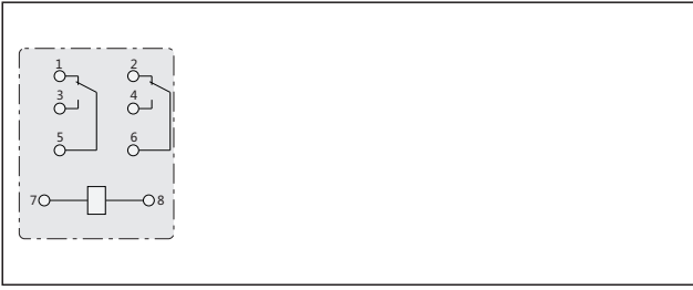
Connection diagram (bottom view) ZZ(D)
