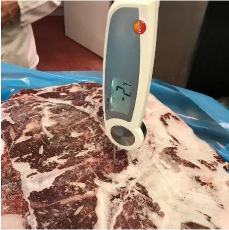
Beef 25% fat, 25 kg 5000 kg/h from -18 °C to -4 °C/-2 °C Block size: 600 x 400 x 260 mm
