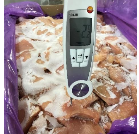
Chicken breasts 15 kg 3000 g/h from -18°C to -4°C/-2°C Block size: 600 x 400 x 260 mm
