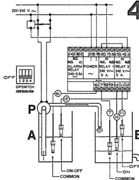
It maintains in **A** the level between the on and off probes and activates the alarm both when the liquid falls below the "low alarm" probe and when it exceeds the "high alarm" probe.
