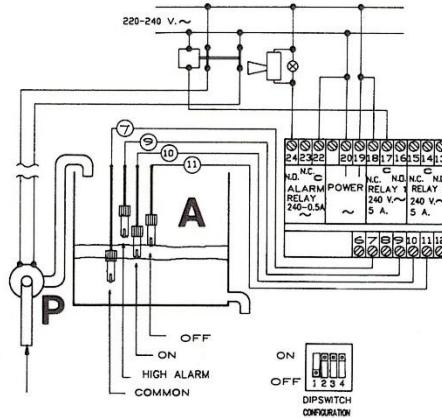
It maintains in **A** the level between the on and off probes and activates the alarm when the liquid falls below the "low alarm" probe.
