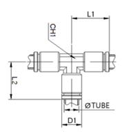
Part No. TUBEL1 L2 D1 CH1 SPE 06 6mm 20mm 20mm 11mm 9.2mm
