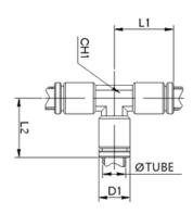
Part No. TUBE L1 L2 D1 CH1 SPE 08 8mm 22mm 22mm 13.6mm 11.2mm
