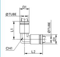
Part No. TUBE L1 L2 D1 CH1 SPV 08 8mm 22mm 22mm 13.6mm 11.2mm
